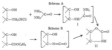
Although the mechanism of this conversion has not been definitely established, it is probable that the urea first breaks down to cyanic acid, which then attacks the basic group with the formation of the intermediate I. Finally, cyclization takes place with the elimination of ammonia. In one case selected for detailed study (5,5-dimethyl-2oxazolidone) it was possible to isolate the intermediate I in good yield and to convert it to the oxazolidone by continued heating.
